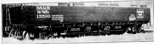
Coal Car, 80,000 Pounds Capacity—C. B. & Q. R. R. Fig. 1.—Showing Johnson Hopper Doors.
